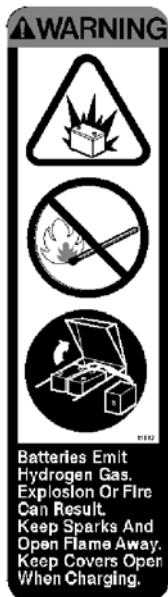
BATTERY CHARGING LABEL - LOCATED IN BATTERY COMPARTMENT AND ON SEAT MOUNTING WELDMENT.
