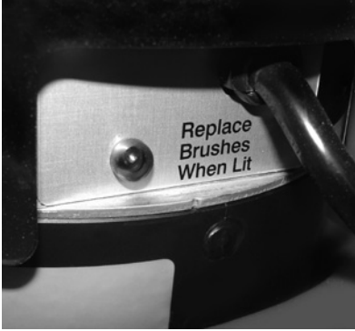
Motor carbon brush wear indicator light alerts the operator to protect the motor.
